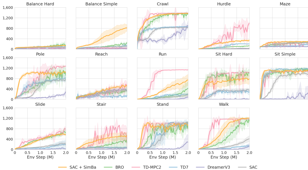
Figure 20: Per task learning curve for HumanoidBench. Mean and 95% CI over 10 seeds for SimBa, 5 seeds for BRO, TD7, and SAC, 3 seeds for TD-MPC2 and DreamerV3. We no
